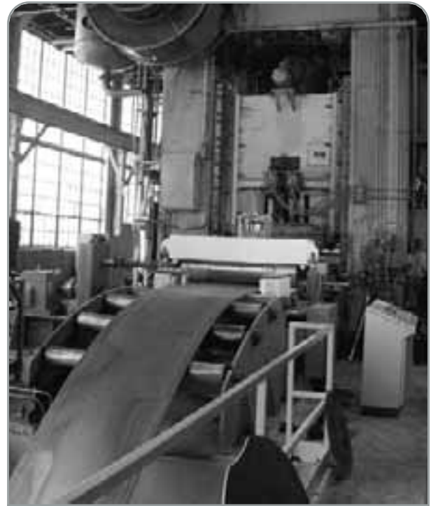
The decoiler feeds steel in one long continuous strip to a 2000 ton press.
