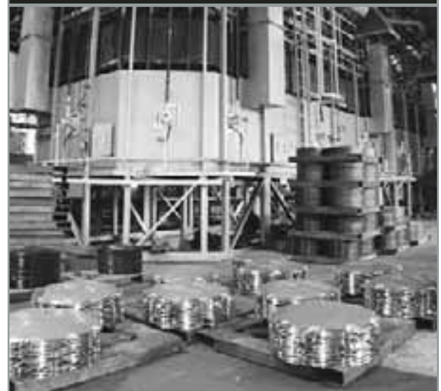
Large capacity furnace heats disks to achieve optimal hardness, without sacrificing ductility.
