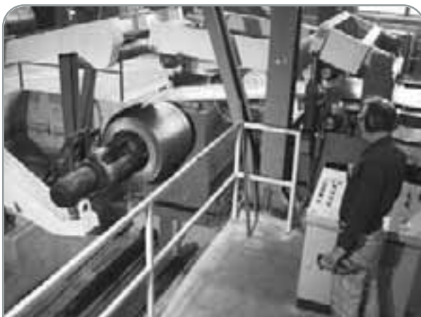
Coils are mounted on decoiler.
