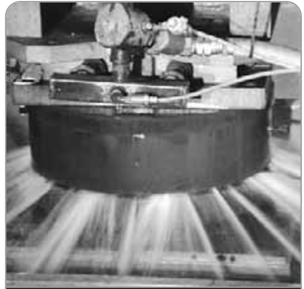
Disks blades are water quenched, firmly locked in their dies, to maintain accurate shape.
