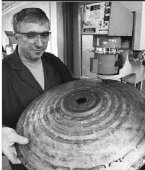
Quality control technician tests disks for hardness.
