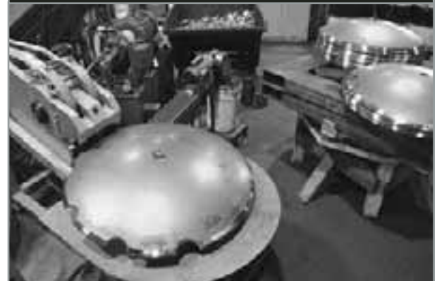
Automatic notching machines can be programmed to produce any required number of notches.
