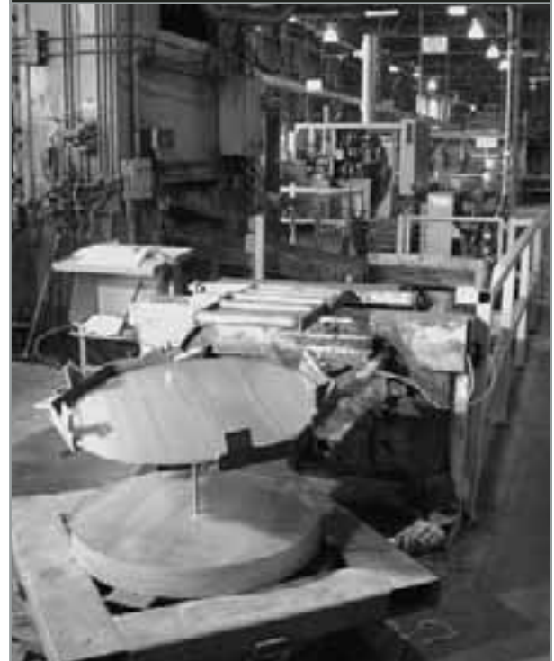
Disk blanks emerge from the press.
